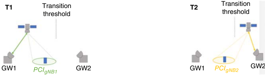
Figure 6.10 “Hard” feeder link switchover for non-geostationary satellites. Source: 3GPP TR 38.821 [11]/The TR is from 3GPP.
