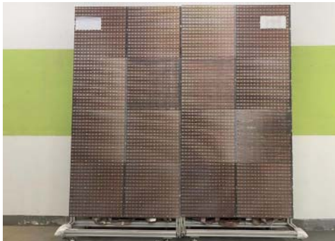
Figure 12.5 The IRS is formed by a 4 \times 4 array of reflecting tiles. Each reflecting tile is 50 \times 50 cm large and consists of 16 reflective elements.
